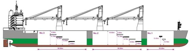
Adjustable tweendecks, box shaped. Unobrstacted deck space 120 x 20mtr
